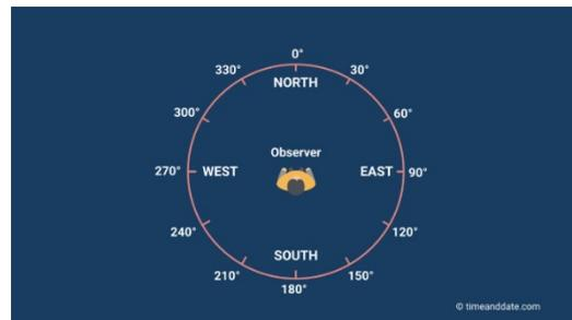
Figure 209: The angle of azimuth explanation (Bikos, 2023)
