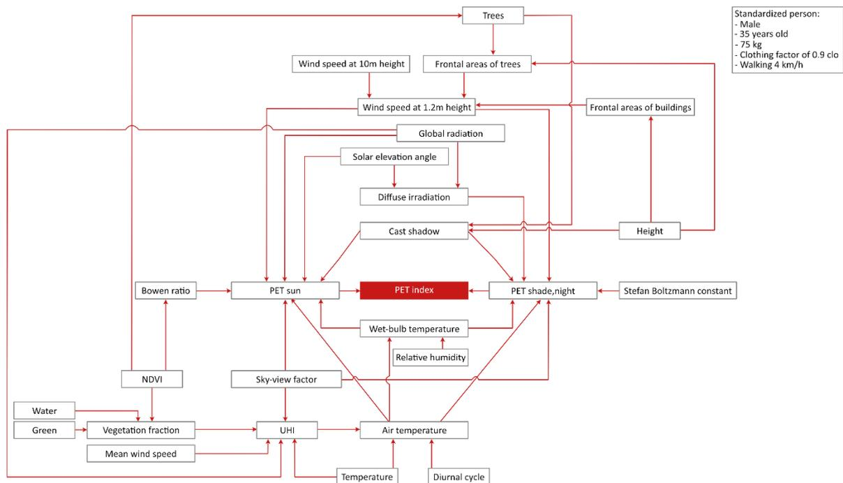
Figure 6: Factors of PET index calculation
