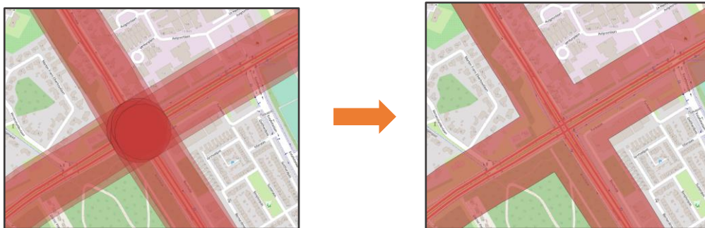
Figure 14. An example of dissolving the overlaid road buffer at the intersection location
