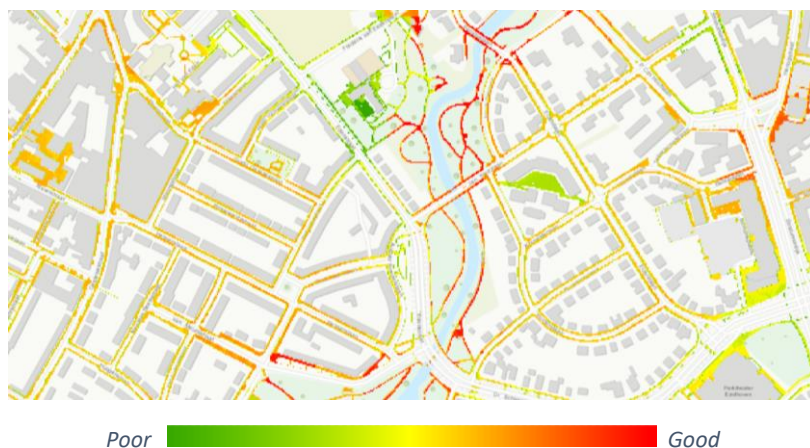
Figure 24. Output WI map at footpath scale after clipping the raster map with footpath polygons in ArcGIS Pro.
