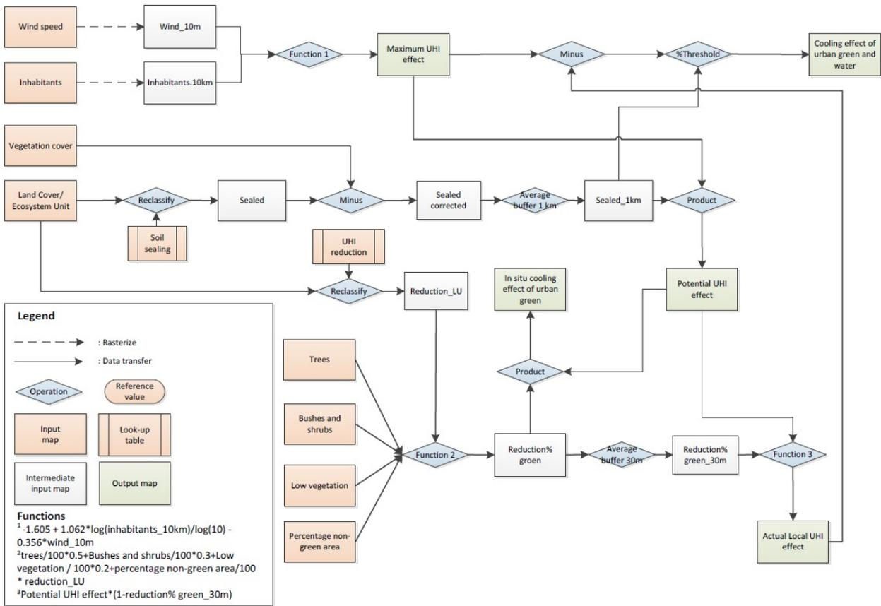
Figure 3.3: Schematic overview of UHI model, taken from [107]
