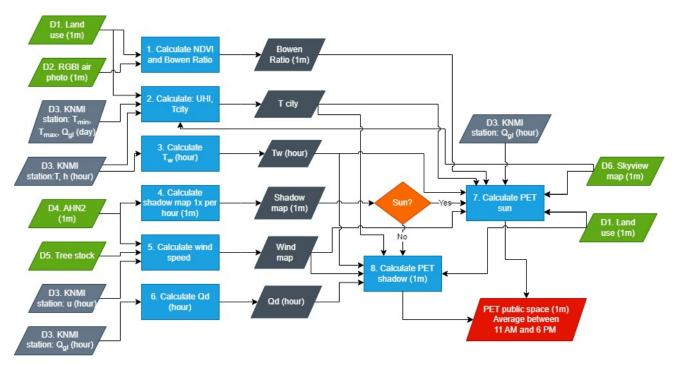
Figure 3.4: Schematic overview of PET model, based on [92].
