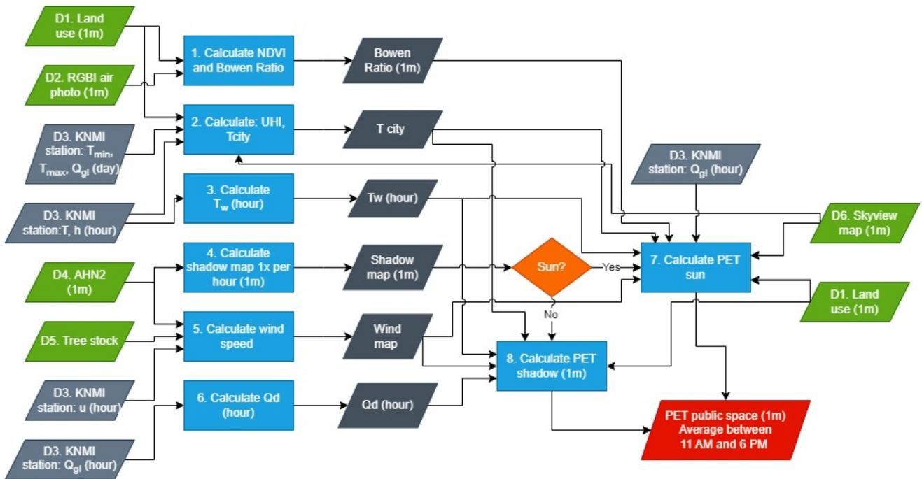
Figure 3.4: Schematic overview of PET model, based on [92].
